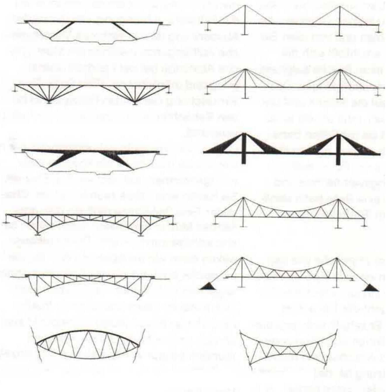
And yet another aspect comes into play. He makes a distinction between in compression-stressed structural members (arches) and tension-stressed members (cables, suspension structures).
