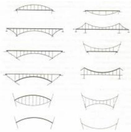
fig. 4: Systematics of Jörg Schlaich: Stiffness by use of bending and pre-stressing from Schlaich
