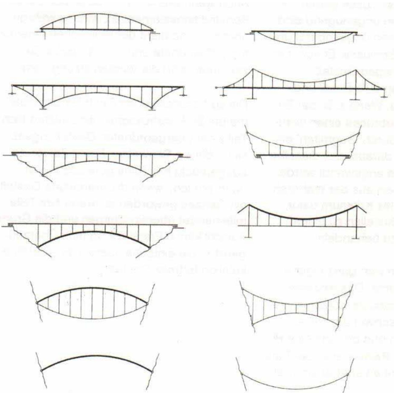
This takes us to Antonio Gaudi who impressively verified and implemented arch/vault as the reversal of cables/cable meshes. Gaudi had hung up chains, lit them candles from below, made drawings and built corresponding arches. This whole method is indeed structurally correct and was known by Leon Battista Alberti, Italy and used in modern times by Heinz Isler, Switzerland.
