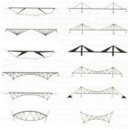
fig. 3: Systematics of Jörg Schlaich: Stiffness by use of trusses and pre-stressing from Schlaich
